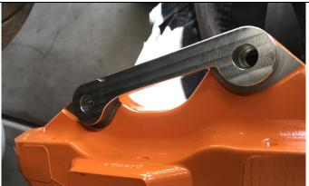
Place the bracket adapter on the caliper and line it up with the knuckle. Adapter is designed to go between the caliper and the knuckle. Slide the supplied 17mm bolts with washer from the back through the adapter into the caliper's thread. Mount the bolts into the caliper. Take care to ensure that the caliper is square and evenly started on both studs. Check for rotor clearance and make sure it's well center on the caliper.
