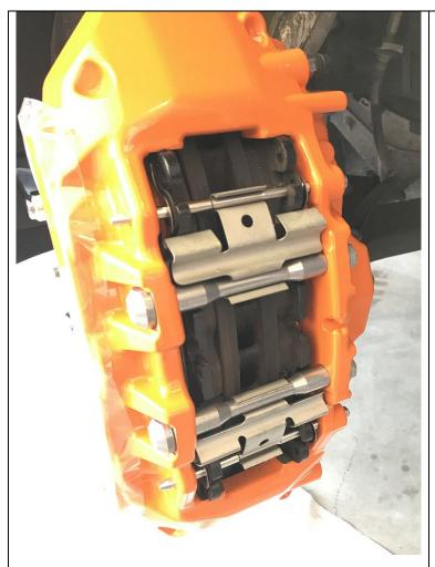
Installation brake pads can be done before or after the caliper is installed onto the car. Slide on the brake pads into the caliper with the warning indicator facing the outside of the car. Take care and ensure that the friction side of the pads is facing the rotors. Slide the pin and retaining clip into place and then tap the pin into its seat from the back side. Picture to the left shows the pads properly installed into the caliper.
