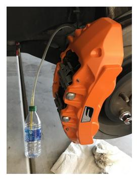
Because you're only installing front brake calipers, you will only be needing to bleed the two front brakes. Start with the passenger side first then the driver side.
