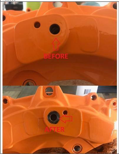
\*Tips: Make sure the area around the banjo bolt is clear of any paint or powder coating. This area must be flat to ensure the seal of the crush washer. With powder coat finish not being flat as possible, there can be possible leaks in the brake lines.
