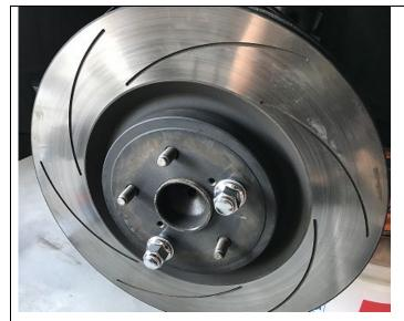
Install the rotor onto the hub. Tighten lug nuts to hold the rotor on to the hub. Rotate and spin the rotor and make sure the dust shield is not hitting the rotor. Picture to the left shows Driver side rotor installed.
