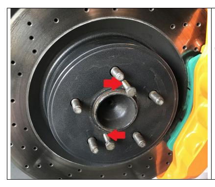
If the rotor doesn't come apart, use two M8x1.25x30 bolts from the hardware store and insert it into the two threaded holes of the rotor's top hat. Screw this down until the rotor comes apart from the hub.
