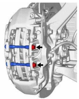
Torque the two brake pad guide tie rods with the two bolts to 30 N\*m (306kgf\*cm, 22 ft-lb)
