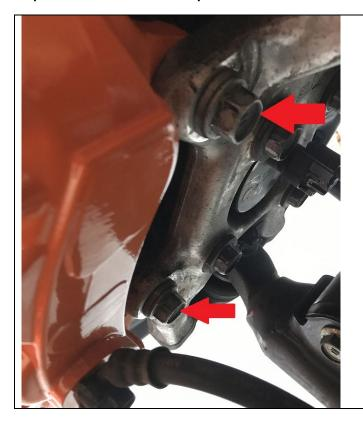
Removal of the 17mm bolt on the IS F brake caliper and leave the caliper aside by hanging or hooking it onto the suspension. Do not remove the brake line.
