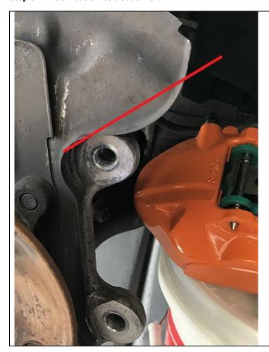
Cut a section of the dust shield off as shown in the red line. That picture on the left is the driver side front dust shield. Use some paint to cover up the section that was cut if needed.
