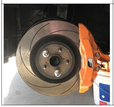
Picture on the left shows installed GS F/RC F Brembo calipers and rotors on driver side.
