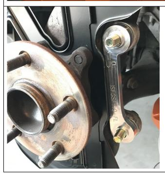
Picture on the left shows the view of the adapter positioned correctly without the caliper and rotor. Position the caliper adapter UP. Picture below shows the adapter installed with the caliper on the knuckle.
