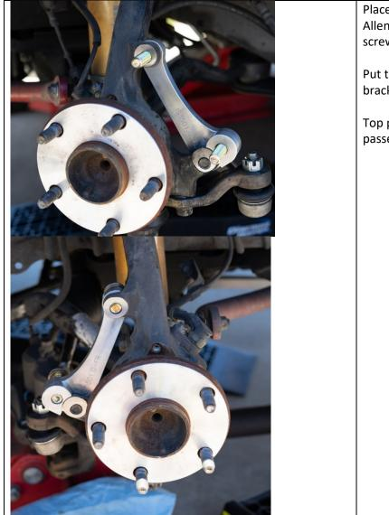
Place the bracket on the knuckle and use the M14 Allen Hex bolt with washer from the backside and screw it through the hole you freshly tapped.
