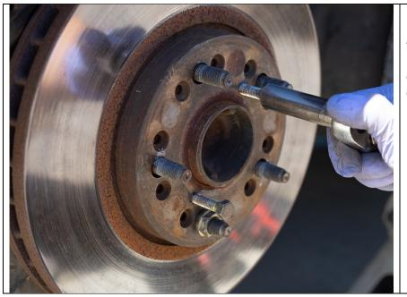
Use the two M8x1.25x30 bolts from the hardware store and insert it into the two threaded holes of the rotor's top hat. Remove any lug nuts or spacers on the lugs of the hub. Screw this down until the rotor comes apart from the hub.
