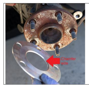
IS350/GS350 4 pot calipers: Install the shim onto the hub with the chamfer side towards the hub. Then place the brake rotor on top of the shim. Rotate and spin the rotor to check for clearance.
