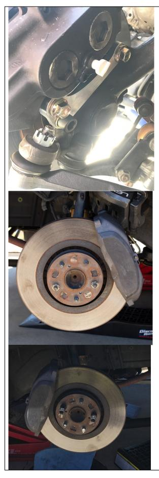
Rotors must be cleaned with brake cleaner. Not doing so will damage the rotors and pads and will prevent the brakes from performing properly.
