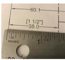
2.Check dimensions both vertically and horizontally to confirm it has been printed to scale.
