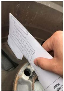
6.Verify that the edge of the caliper does not touch the rim or the wheel spokes. A minimum clearance of 2mm (0.080") is recommended.
