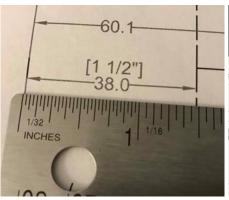
2.Check dimensions both vertically and horizontally to confirm it has been printed to scale.
